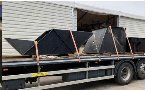
Chute sections to make up a full arrangement ready for site service installation.
