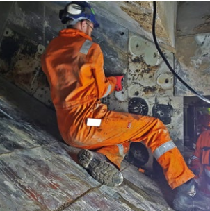
Removal of worn liner plates
