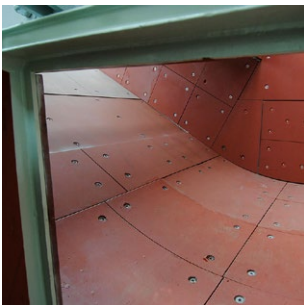
Replacement liner plates within the submerged ash extractor
